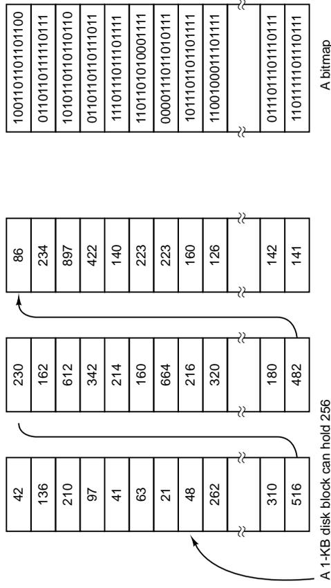
A 1-KB disk block can hold 256 32-bit disk block numbers
